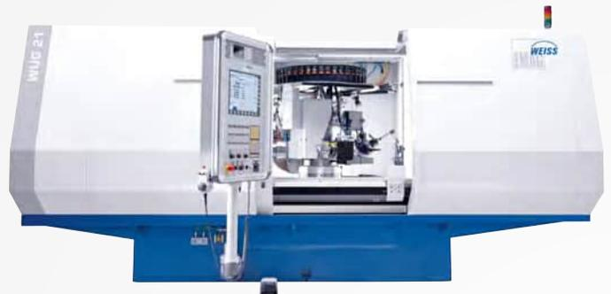
Manual or fully automatic? The WUG 21 CNC universal cylindrical grinding machine means that you do not have to decide on one or the other as you can switch between manual or fully automatic grinding at the touch of a button. As a result of these features and the wide range of equipment, the WUG 21 cylindrical grinding machine is the ideal machine for small series, single parts, and prototype production.
