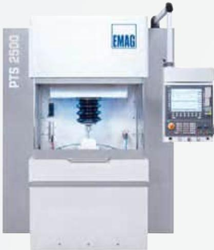
The economical solution for PECM process development and for the PECM machining of challenging 2D and 3D geometries.
