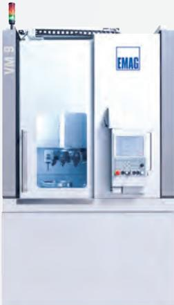
The vertical turning centers in the VM Series are designed for the highly productive manufacturing of workpiece families with a wide range of parts. A tool turret with twelve tool positions, depending on the required tool interface in a BMT or VDI version, is available for machining. The turret can be equipped with driven tools to carry out drilling operations, for example.
