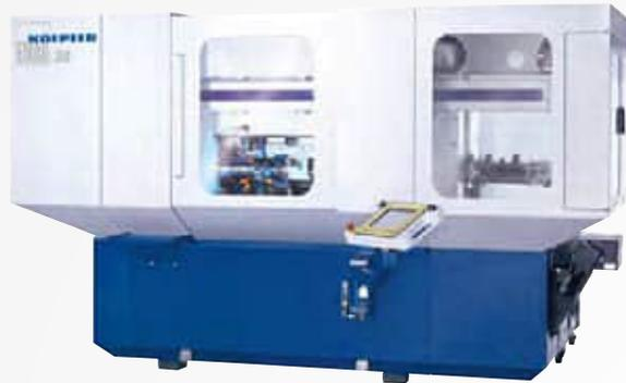
The K 300 hobbing machine is a fully automatic machine with nine activated CNC axes to allow the flexible machining of gear wheels up to module 4.
