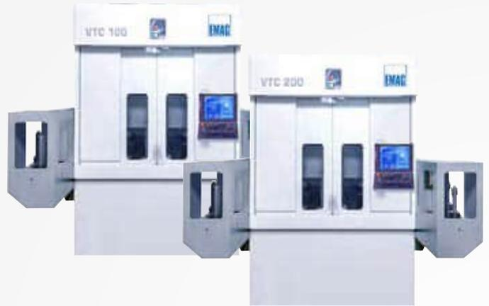
The strength of the VTC Series machines is their 4-axis machining of large quantities of shafts up to 400 mm in length. Since the machine concept comprises a fully integrated automated loading and unloading system, a manufacturing system can be created, which features very short transport distances. The machines are loaded and unloaded by the two turrets, which ensures that the process is fast and straightforward.
