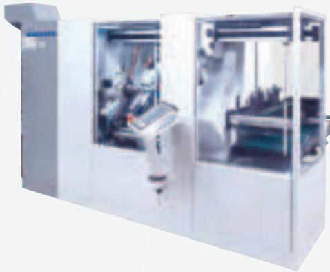
The K 160 hobbing machine features the very latest generation of control systems and can provide high speeds at its milling head and main spindle.
