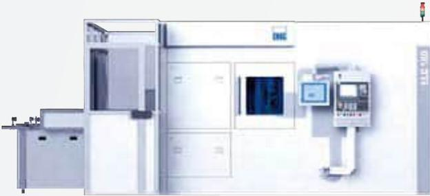
The ELC 160 is a modular system concept, which can be configured for a wide range of tasks. The ELC 160 can be fitted with all laser technologies. Whether you are using a CO<sub>2</sub> laser or fiber-guided systems (fiber, disk) – anything is possible.
