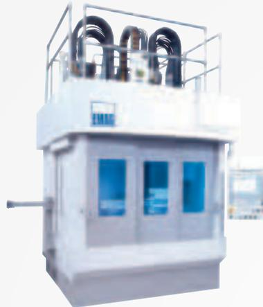
The perfect machine for machining demanding shaft-type workpieces – vertical turning and/or grinding.
