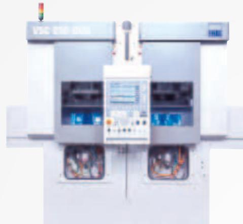
The low-cost solution for machining small and medium workpieces in two operations. The DUO design has two separate machining areas, which means that it has overhead slides that can be programmed independently.
