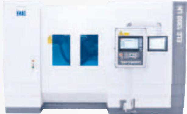
The ELC 1300 LH is a production laser hardening machine developed for laser hardening shaft-type workpieces such as special tools with HSK interfaces. The machine design with an NC moving lens minimizes the programming work for new workpieces. This means that the machine can be very easily retooled to handle a very wide range of workpieces with similar hardness values.
