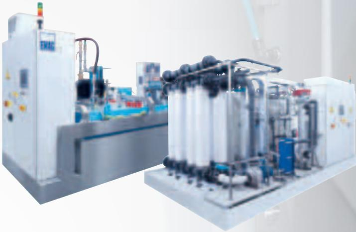
Both systems with chamber filter presses and with micro-filtration are available for filtration purposes. The filtrate quality and volume can thus be tailored precisely to requirements. Systems from 40 to 900 l/min filtration capacity are available as standard.
