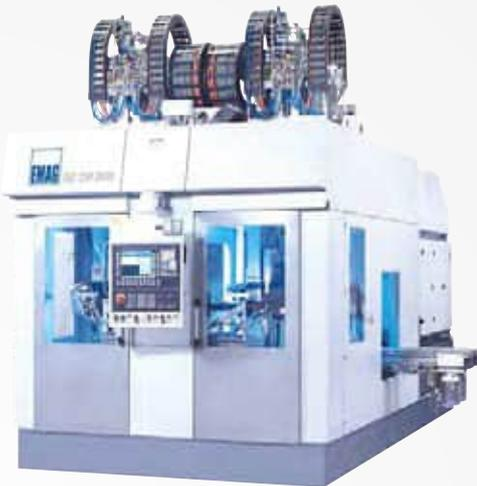
The ELC 250 DUO uses the pick-up principle – its spindle loads itself using the pick-up method and positions the workpiece for the welding lens or other process modules.
