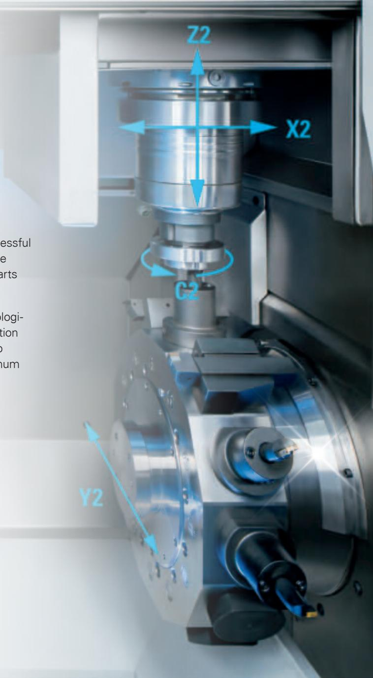
EMAG has extended the product range of the extremely successful VL Series in the form of the VL 3 DUO, a twin-spindle machine solution for the highly productive manufacturing of chucked parts with a diameter of up to 150 mm.
