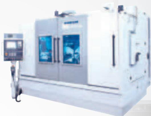
The HG 208 DW four-axis grinding machine for simultaneous machining can complete two external grinding operations on shaft-type workpieces at the same time.
