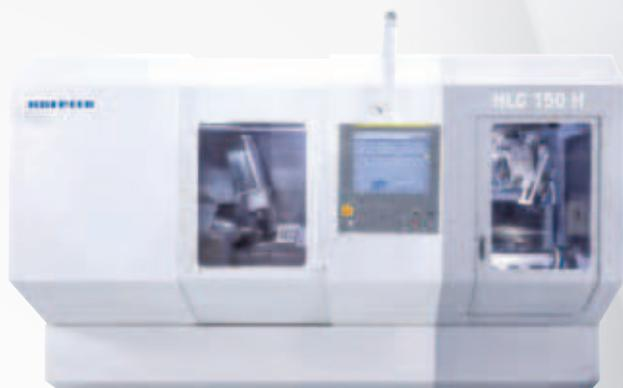
The HLC 150 H, the most modern horizontal hobbing machine available from EMAG KOEPFER, is a universal solution for hobbing and skiving, as well as worm milling and skiving processes, for components up to module 3.
