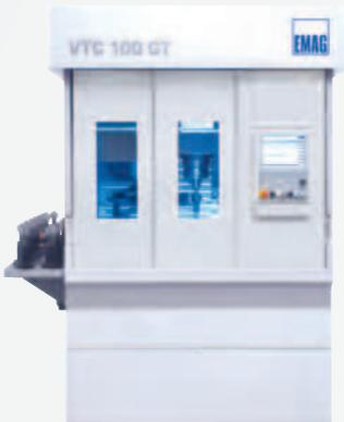
Versatile solutions for shafts: The VTC 100 GT ensures a quick process for hard turning and grinding. The tool turret completes all turning operations and the workpiece loading work. A powerful grinding spindle is available for precision external cylindrical machining. This can be fitted with both CBN and aluminum oxide grinding wheels.
