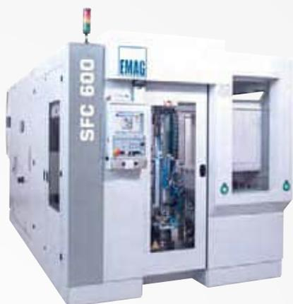
The joining machine SFC 600 features our patented thermal stress-free joining process combining precision and high flexibility for the heat shrinking of components (cams, bearing rings, sensor wheels, etc.) onto camshafts.
